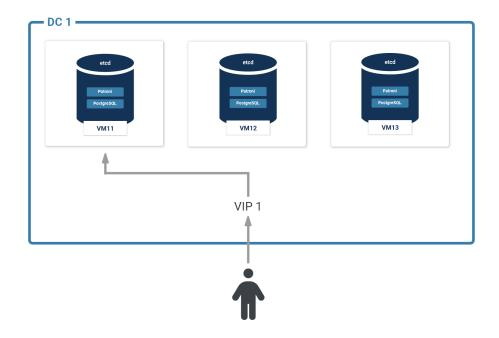
Patroni will ensure that there is always **one active node** which can be used to **"read / write"** operations. All other nodes are standby systems and are only available to read data and are therefore suitable for load balancing.
