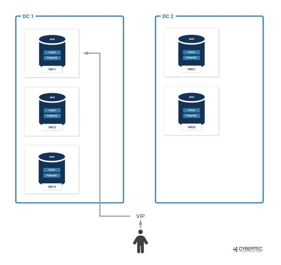
The secondary data center could be modified to run on its own if a new etcd cluster is created in the secondary data center. This could serve as an emergency fallback but requires a bit of time to configure in case of such an emergency.
