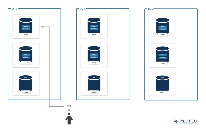
Any data center (or any link between the data centers) can fail; As long as two data centers can still communicate with each other, quorum can still be reached and the PostgreSQL service is still writeable.
