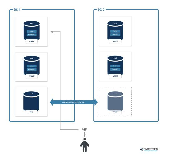
Subsequently, when the primary datacenter is unreachable, the hypervisor could decide to run the **replicated VM in the secondary datacenter**, thus enabling that secondary datacenter to reach quorum.
